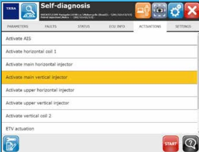
3. Navigation within the software screens is easier thanks to the use of tabs (PARAMETERS, STATUSES, ERRORS, ECU INFO, ACTIVATIONS, ADJUSTMENTS).
