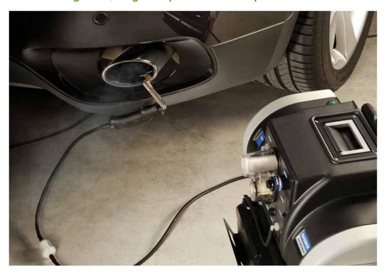
For the checks connected to anti-pollution regulations, TEXA offers tools such as GASBOX Autopower (exhaust gas analyser for petrol and gas vehicles), OPABOX Autopower (opacity meter for diesel engines), MULTI PEGASO 3 (analysis station with a LED monitor), RC2 and RC3 (rev counters for cars and trucks), RCM (rev counter for bikes).
