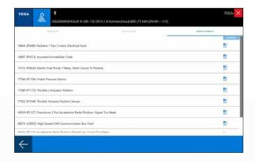
After performing a global scan of the control units on board the vehicle, the Guided Diagnosis tab shows any detected errors and allows launching the troubleshooting procedure by clicking on the specific icon.
