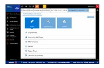
The new HaynesPro database, consisting of the Tech, Electronics and Smart modules, is easy to use and accessible from the Technical Data and Checks menu item, but also from the TGS3s vehicle scan and from the diagnostic system via a direct link.
