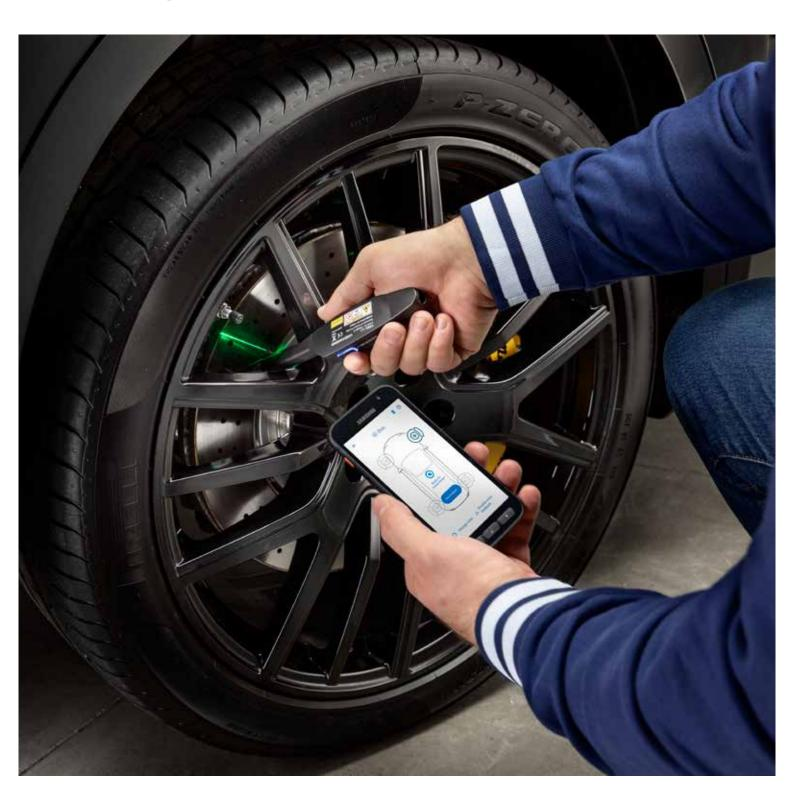
TEXA's new product in the field of measurements is **LASER EXAMINER**, a laser profilometer to check brake disc and tyre tread wear. TEXA's **UNIProbe** and **TwinProbe** interfaces allow taking all the physical measurements required for a conventional diagnosis, identifying potential faults. On the other hand, TTC (TEXA TENSION CONTROLLER) is ideal for the correct tensioning and mounting of the timing belt on bikes, ensuring an extremely professional service.
