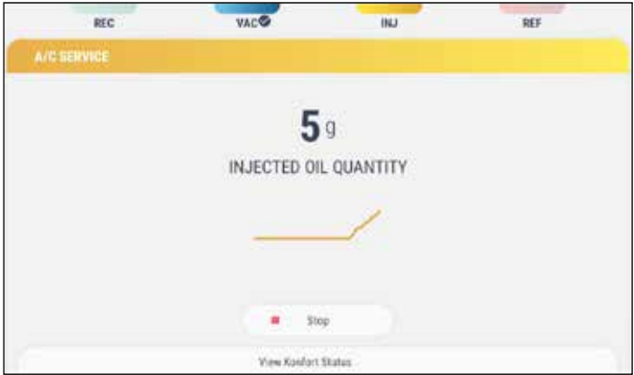
«Oil injection» phase: the system injects the correct amount of oil in the vehicle system to lubricate it.
