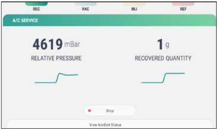
«Recovery» phase: the screen highlights the time remaining until the refrigerant recovery operation is complete.
