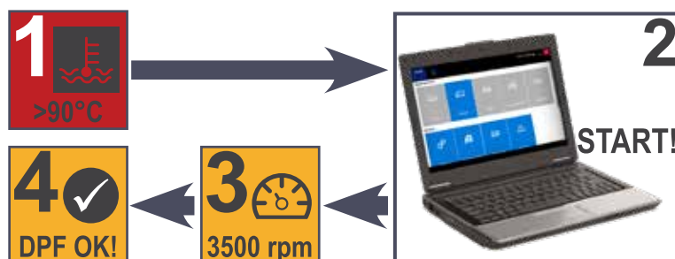
Figure 124: Operation sequence for forced regeneration
