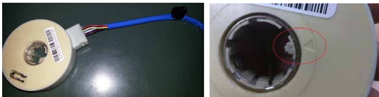
Figure 108: Angle Steering sensor. Point "0" detail useful for the centre setting of the sensor.
