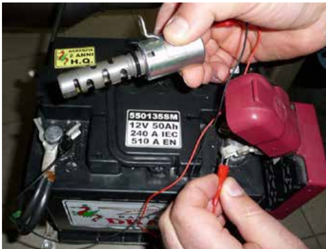
Figure 98: OCV valve disassembled and connected directly to the power supply 12 V
