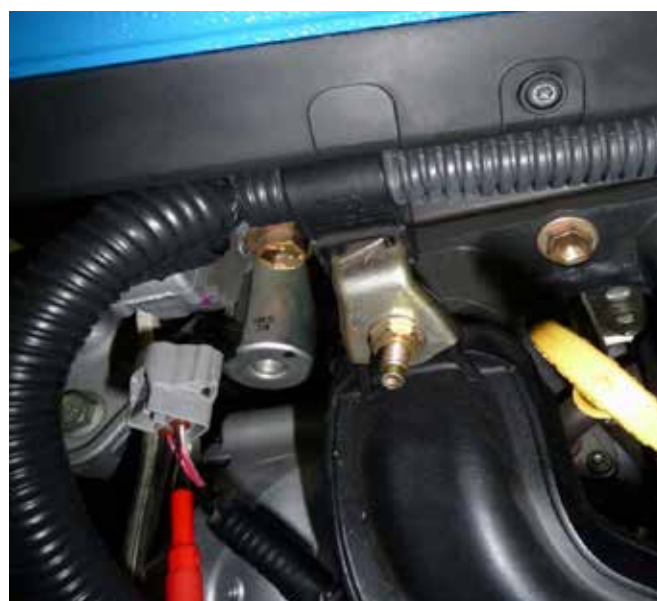
Figure 96: Oscilloscope settings on the OCV Solenoid Valve
