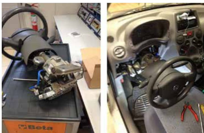
Figure 109: Disassembling procedure of the EPS assembly
