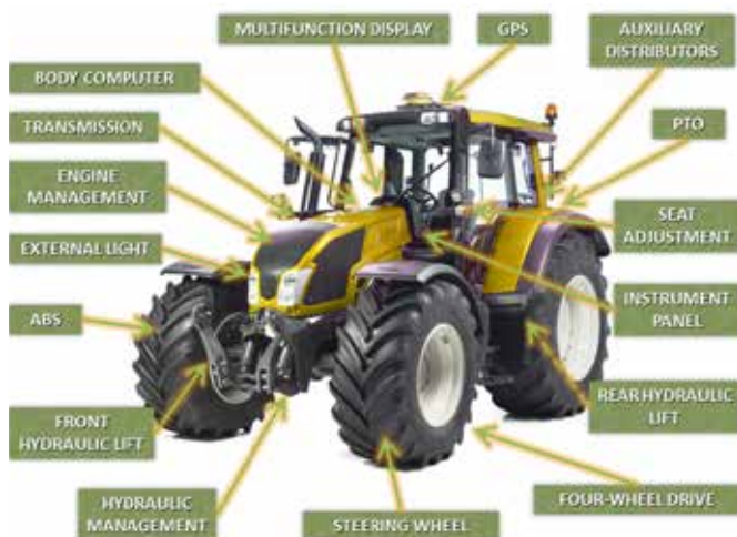
Figure 42: Electronic systems in Off-Highway vehicles
