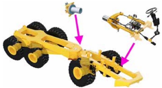
Figure 17: Articulated dump truck chassis structure
