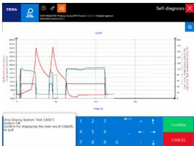
Figure 97: "Urea Dosing System Test (UDST)" diagram
