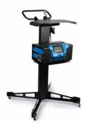
Measurement of particle number concentration (PN) in the exhaust of motor vehicles has recently become really important in several European countries and it will be integrated in PTI legislation starting from Netherland, Belgium and Germany. Charge-based sensing techniques for the examination of PN, like Diffusion Charging (DC), represents the main technology available for this type of check.
