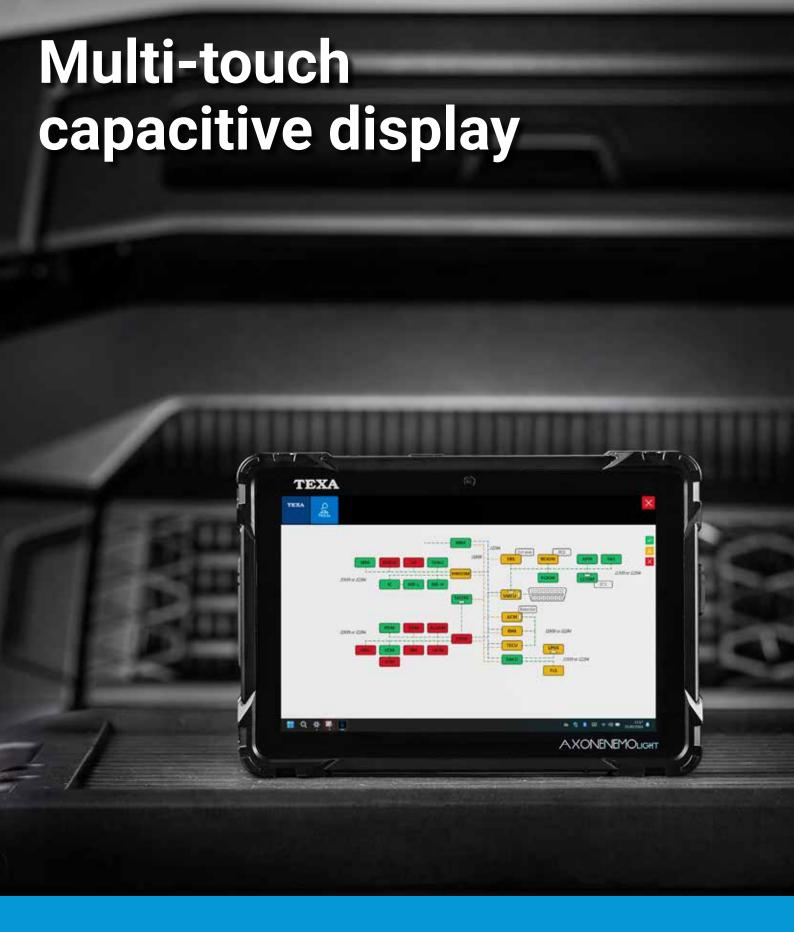
Thanks to the 10.1" high-contrast multi-touch capacitive display with a 1920x1200 pixel resolution, AXONE NEMO LIGHT offers an extraordinary useability and a detailed control on all the operations that must be completed.
