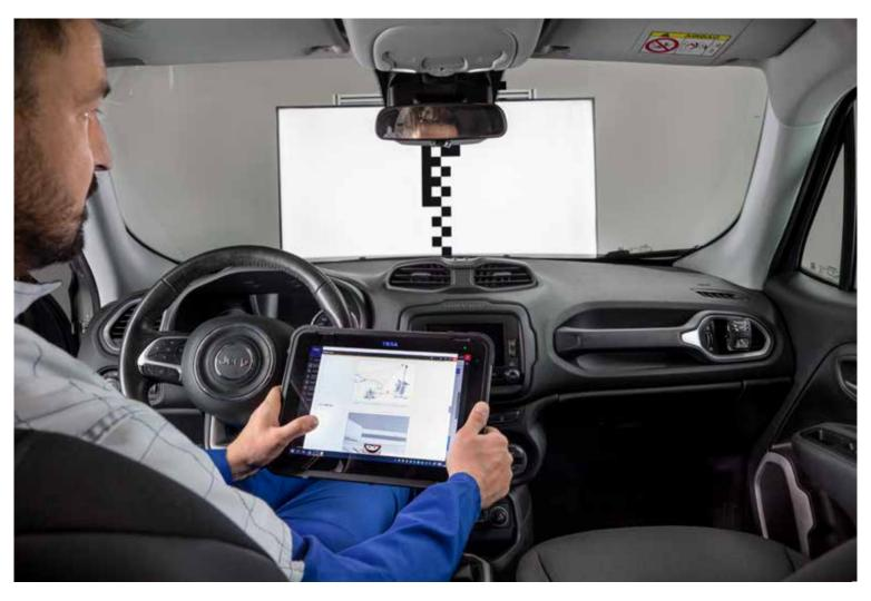
The **images** of the panels are transmitted and **positioned automatically**, based on the vehicle selection made. They are displayed through a linear, safe and quick process.
