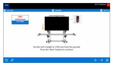
The unit must be moved electrically in order to position it at the correct height.
