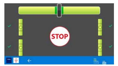
The 4 CCD detectors must be parallel to the work surface and the steering must be centralised. When these conditions are achieved, the display reads out "STOP".
